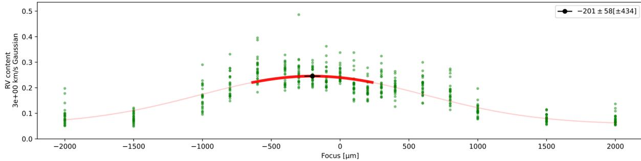
Figure 10: Through focus measurements before detector integration (Room temperature, April 2022, La Silla)
