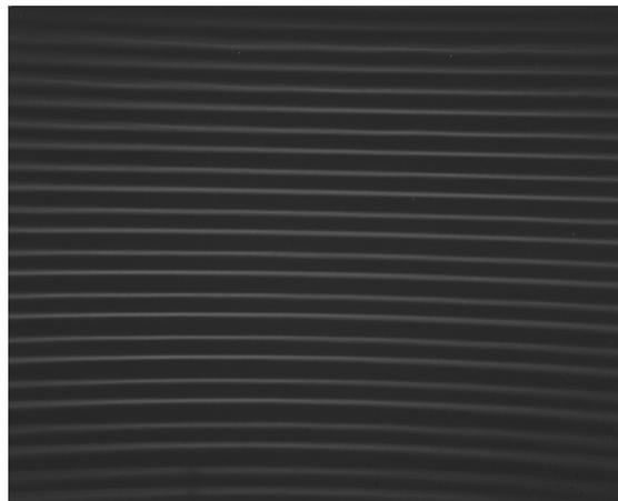
Figure 8 Flat on C-Red2 (room temperature)
