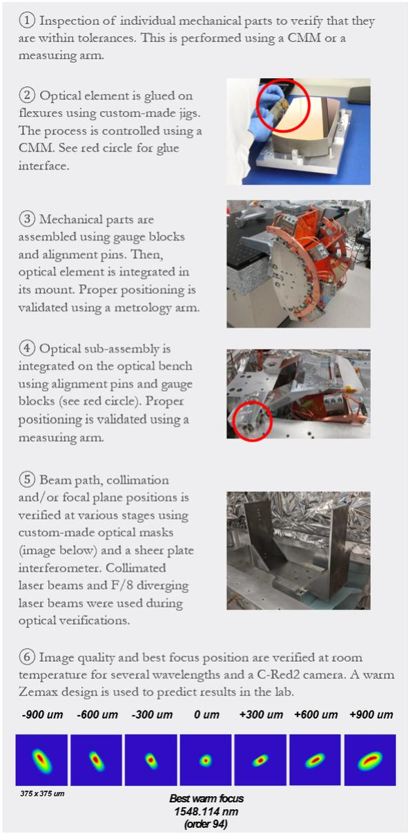
Figure 6 Room temperature integration and test flow
