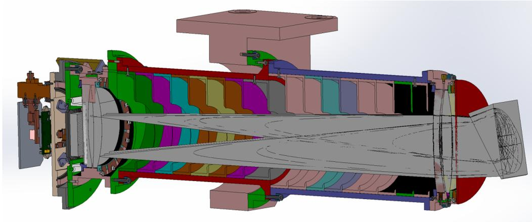
Figure 4. Camera mechanical cross section (detector left).
