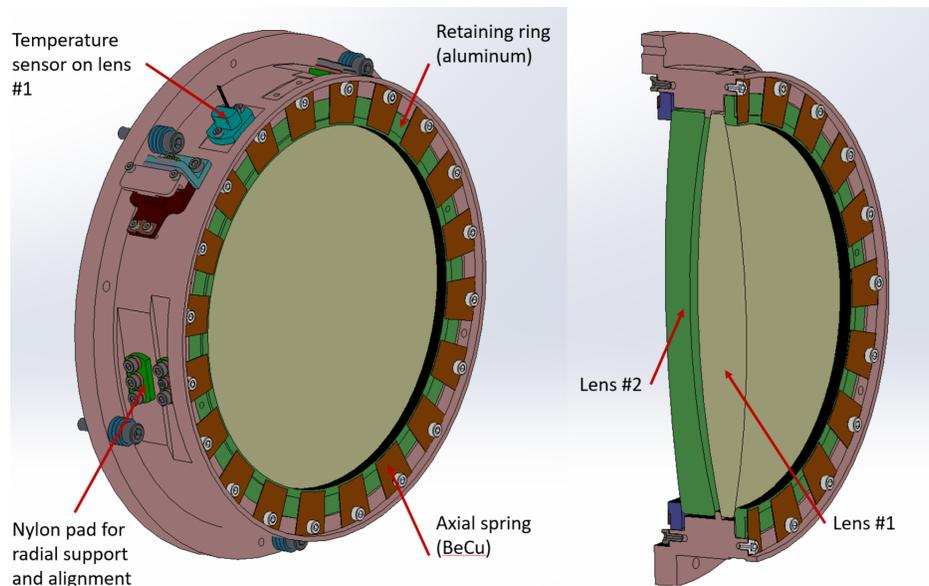
Figure 5 Camera lens cell assembly
