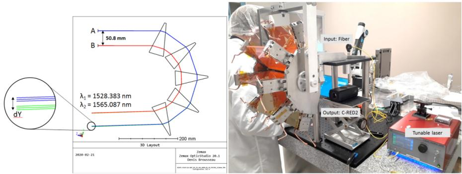
Figure 7 Setup to test the prism carousel (left: zemax layout, right: setup)
