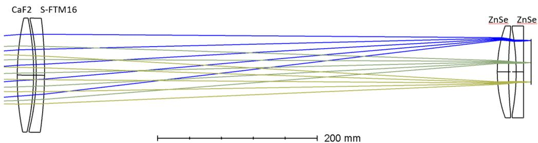
Figure 3. NIRPS spectrograph camera layout.(detector right)
