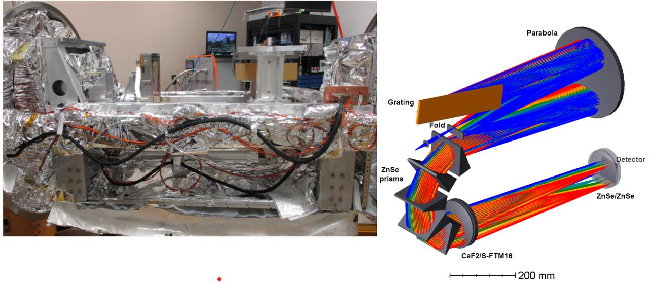
Figure 2. NIRPS spectrograph (Left: Instrument view, parabola at left, grating and injection at right, camera and detector underneath,; Right: optical layout.)
